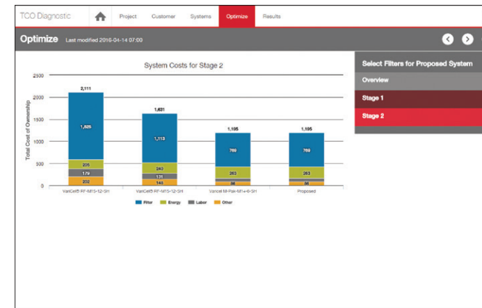
This depicts filter cost optimization relative to annual costs for filters, energy, labor, and other total cost of ownership for the Current System, two Optimized Options, and the Proposed System.
