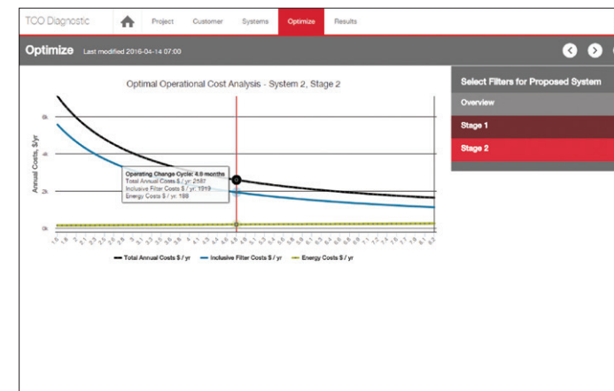
Service Cycle Optimizer allows the user to adjust the service cycle and see the values for total cost, energy cost, and filter cost change.
