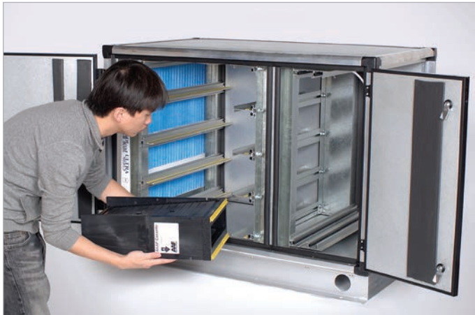
Step 1: Prepare to install the half-cassette. Address the air outlet side sealing track at a slight angle as shown.
