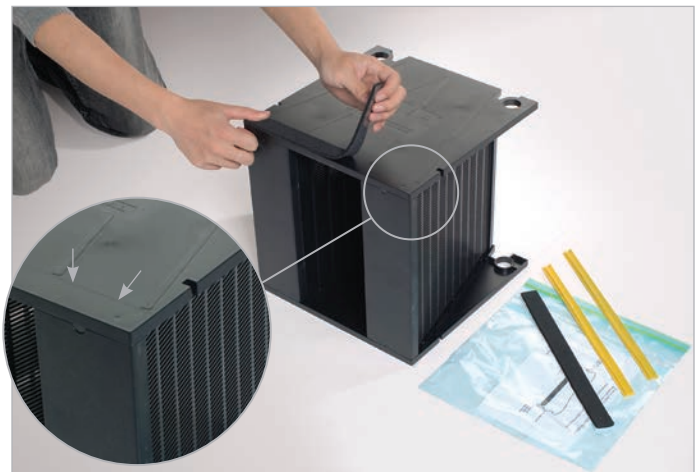
Step 2: Locate the gasket on the leaving air side of the half-cassette along the edge of the cassette side plate. A gasket location guide has been formed into the side plate. The gasket should be located to the outside of this line.
