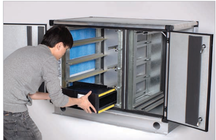
Step 3: Rotate the cassette slightly so that the vertical locator bars are inserted into the slots in the half-cassette while maintaining the compression between the hollow core and butterfly gaskets. See Detail 1 – Step 3 and Detail 2 – Step 3.
