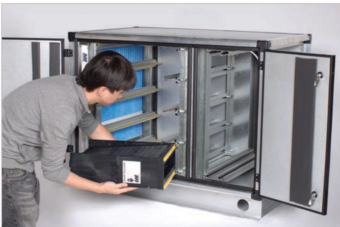
Step 2: Engage the upper and lower black hollow core gaskets in the tracks with the yellow butterfly gaskets on the half-cassette, see Detail – Step 2. Also, begin to align the upper and lower notches in the half-cassette with the vertical cassette locator bars which form part of the track.
